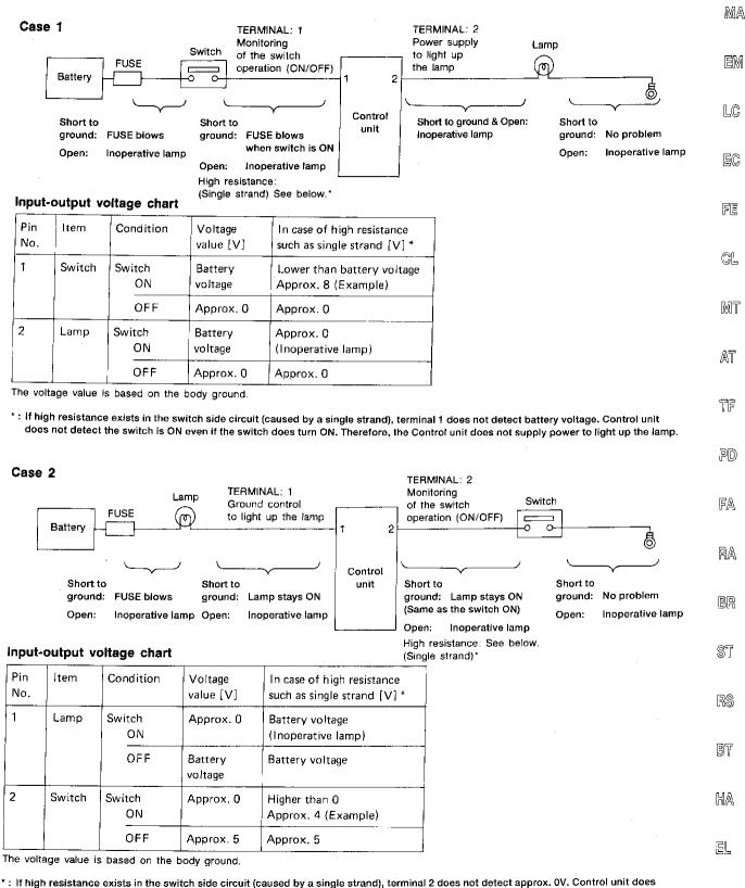
not detect the switch is ON even if the switch does turn ON. Therefore, the Control unit does not control ground to light up the lamp.
