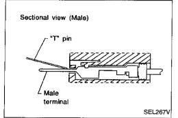
Carefully probe the contact surface of each terminal using a "T" pin **Do not bend terminal**.
